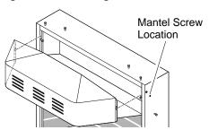
Figure 12 - Removing Hood
